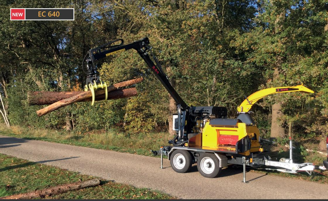
UP TO 70 M3/H. UP TO 200 HP UP TO 400 MM LOGS.
